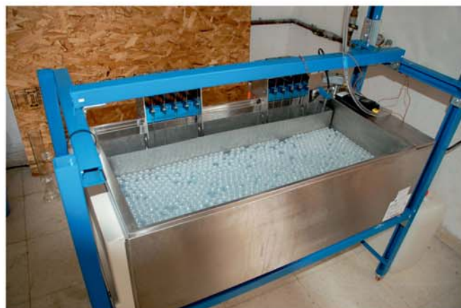
Equipment of stress-cracking determination (source: CETEC)
